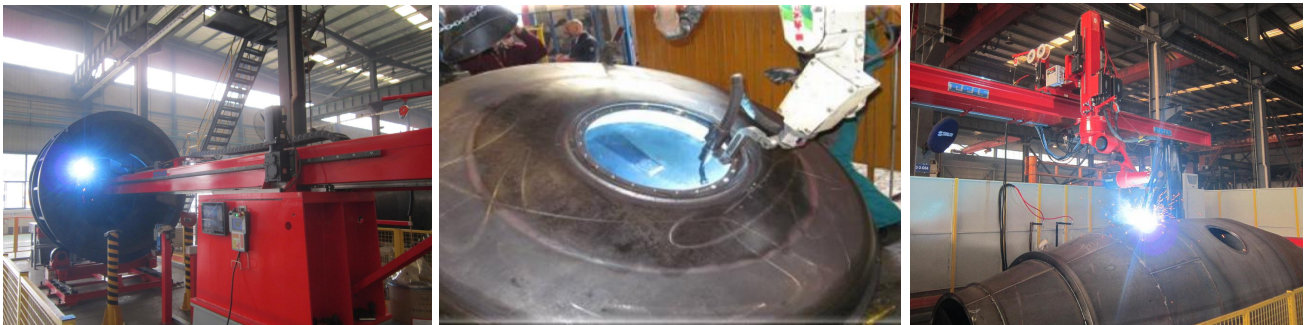
自动机器人焊接搅拌筒筒体 Manipulators solder the mixing drum
